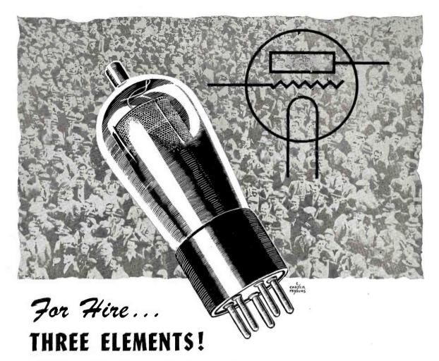
This is an odd-looking symbol that resembles a circle enclosing a hair pin, a zig-zag and a pan-cake turner. However, it's the electronic engineer's symbol for the vacuum tube such as you use in your radio. The three elements in the circle are called,— the filament, grid and plate. The purpose of the vacuum tube is to detect and amplify incoming signals.
