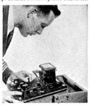
Loran (short for LOng RAnge Navigation) uses radio waves which hug the earth's surface instead of going off into space. Two sets of stations, about 300 to 400 miles apart, send out impulses to a Loran receiver on shipboard like the one shown above. It then shows the ship's exact position.
